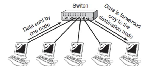
By forwarding data only to the connection that should receive it, the switch can improve network performance in two ways. First, by creating a direct path between two devices and controlling their communication, it can greatly reduce the number of collisions on the network. As you might recall, collisions occur on Ethernet networks when two devices attempt to transmit at exactly the same time. In addition, the lack of collisions enables switches to communicate with devices in full-duplex mode.
